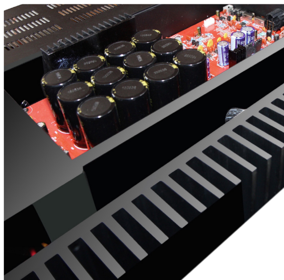
Large heatsink and 12 10,000 \mu F each, or 120,000 \mu F.
