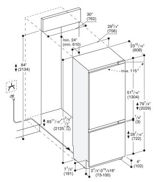
The door face dimensions are designed for a maximum gap of  $\mbox{\em 16}"$  (3 mm).
