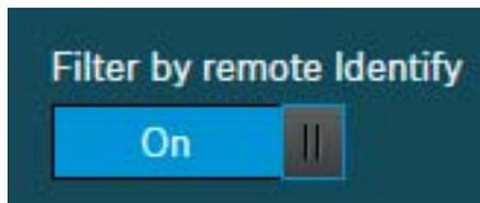
This function allows you to filter the Device List by hardware. This can be helpful when you are in a certain location and want the Device List to display certain devices from that location.
