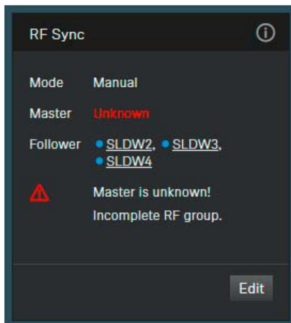
The master receiver is not in the device database of the Control Cockpit.
