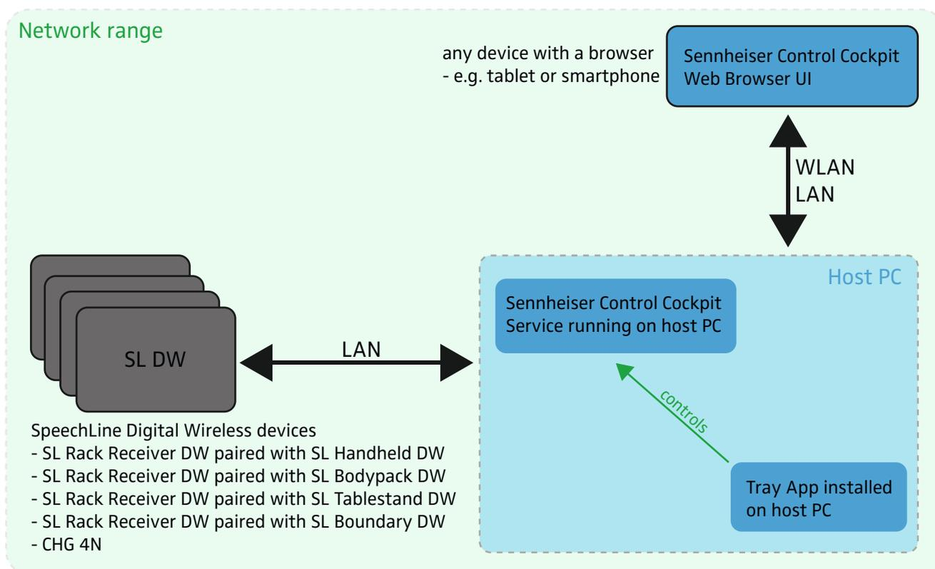
**i** Please note that you only need to install the **Sennheiser Control Cockpit** on **one host PC**. All devices, which are in the same network as the host PC and the SpeechLine Digital Wireless devices, can access the **Sennheiser Control Cockpit** remotely via the **browser-based application**.
