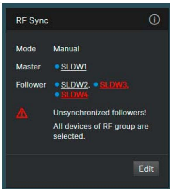
One or more followers in the RF group are not synchronized with their assigned master receiver. This may happen when receivers have an active link and the RF sync settings are changed.
