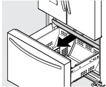
3. Slightly push inward on the basket tabs to release the upper basket from the slide assemblies (one per side, in front).
