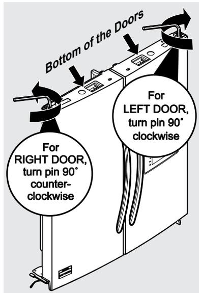
Once you reset the door pins, follow the steps **To reinstall the refrigerator doors**.
