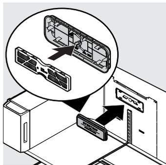
1. Place fingers on bottom of air filter cover and pull from the top toward the front of the unit, releasing the top snaps on the air filter cover from the air tower.
