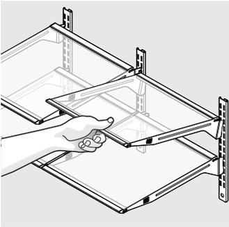
3. Replace by inserting the mounting bracket hooks into the desired support slots.
