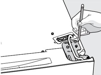
4. Remove the bulkhead cover at the rear of the unit to access the water tube. Disconnect the water tube at the push-lock connection on the rear of the unit below the bulkhead. The dispenser line is connected to the yellow water line coming from the main water valve.
