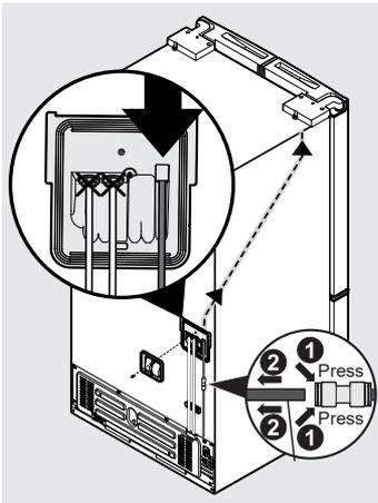
5. Pull the water tube out of the conduit from the top of the cabinet.
