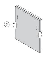
Slide the custom panel up so that the top of the door panel is flush with the control panel.
