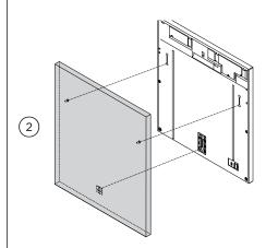
Close the door of the dishwasher and align the screws of the accessory panel into the lower keyhole of the dishwasher door.
