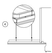
Open the door and remove the four screws and replace with Ø3.9 x 1 1/2" (38mm) screws to fix the panel into place.
