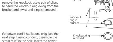
strain relief in the hole. Insert the power cord through the strain relief and tighten. Allow enough slack to easily attach the cord terminals to the terminal block. If tabs are present at the end of the winged strain relief, they can be removed for NOTE: Do not install the power cord
