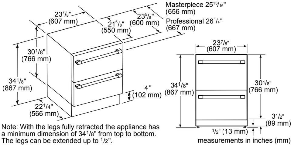
Note: With the legs fully retracted the appliance has a minimum dimension of 34<sup>1/8</sup>" from top to bottom. The legs can be extended up to 1/2".
