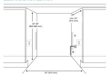
4: Recommended area for installation of power connection – a 2 ½" (63 mm) diameter hole is recommended 3: Location of power cord – approximately 15" (381 mm) from base of appliance
