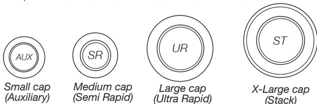
Burner caps should be level when properly positioned. If burner caps are not properly positioned, surface burners will not light. The burner cap should not rock or wobble when properly aligned.
