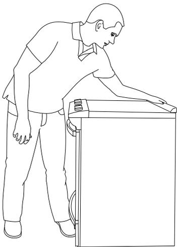
3. Slowly attempt to tilt the range forward. If you encounter immediate resistance, the range foot is engaged in the anti-tip bracket. Go to Step 8.
