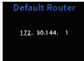
Use this screen to enter the IP address of the gateway router between the PC-300 and management stations that exist on other network segments.
