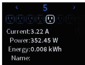
Use the left and right buttons on the Nav Pad to navigate between the eight outlets (the number of the selected outlet is displayed on the top of the screen). The following information is displayed for each outlet:
