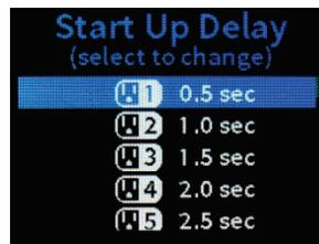
Use this screen to set the time that it takes for the selected outlet to receive power after the PC-300 is powered on (in seconds). Use up and down on the Nav Pad to select an outlet, and then press the center button to select that outlet. An individual **Start Up Delay** screen displays.
