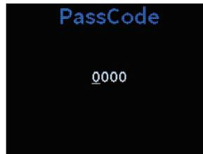
3. The default passcode is "0000." Press the center button on the Nav Pad to enter the code.
