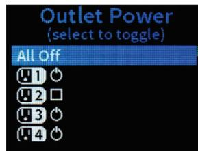
Use this screen to power the PC-300's rear outlets on or off. Use up and down on the Nav Pad to select an outlet, and then press the center button to toggle the power for that outlet. A power symbol (🔌) indicates that the outlet is powered on, while an empty check box indicates that the outlet is powered off.
