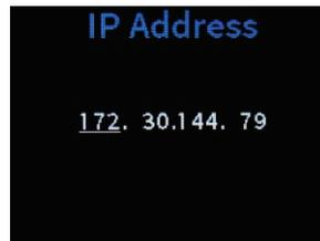
Use this screen to enter an IP address of the VLAN (virtual LAN) interface that is allowed management access.
