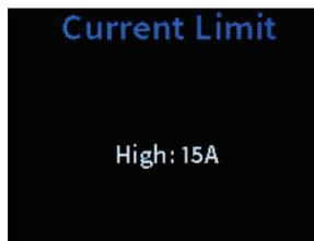
Use this screen to set the overcurrent cutoff, in amperes. The PC-300 shuts off if the combined amperes of the AC outputs are detected to have gone over this number.
