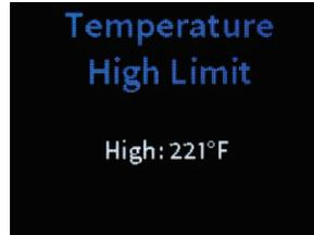
Use this screen to set the temperature cutoff in the selected unit of measurement. The PC-300 shuts off if its temperature is detected to have gone over this number.
