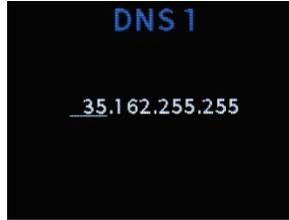
Use this screen to set the primary DNS used to resolve the domain name to an IP address.
