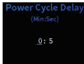
Use this screen to set the duration that an outlet cycles off before powering back on, in minutes and/or seconds.
