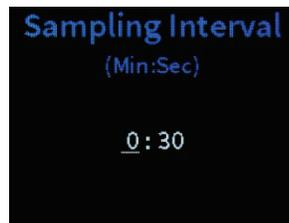
Use this screen to set the sampling interval between the times event logs are recorded, in minutes and/or seconds. (The **Data logging** option on the **Control** screen must be selected.)
