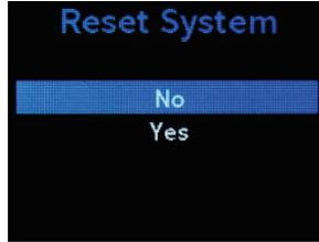
Use this screen to perform a factory reset. Select **Yes** to reset the system. A screen asking **Are You Sure?** displays. Select **Yes** again to confirm the change or **No** to cancel.
