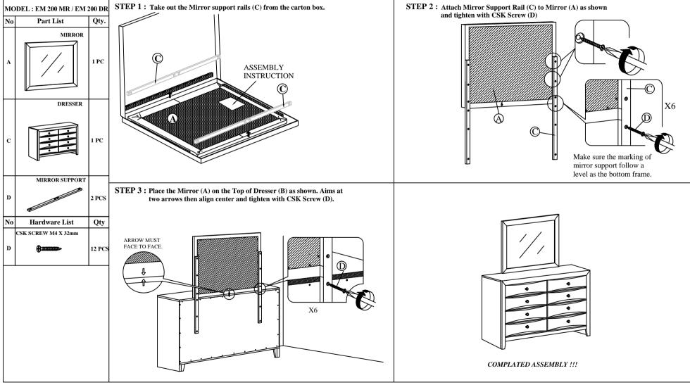
NOTE : SCREWS WILL BECOME LOOSE WITH USE AND OVER TIME WILL NEED TO BE TIGHTENED PERIODICALLY. CHECK TIGHTNESS OF ALL SCREW EVERY 6-8 WEEKS. THANK YOU FOR PURCHASING THIS QUALITY PRODUCT. BE SURE TO CHECK ALL PACKING MATERIAL CAREFULLY FOR SMALL PARTS WHICH MAY HAVE BECOME LOOSEN INSIDE THE CARTON DURING SHIPMENT.
