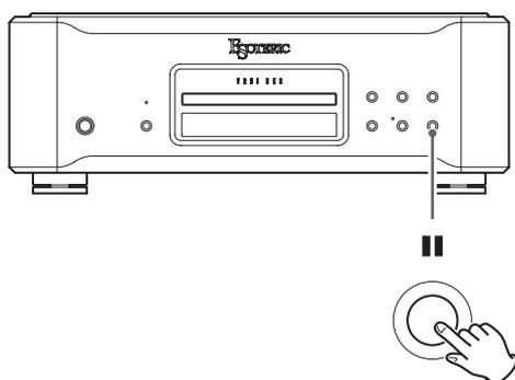
During playback, press the pause (■) button to pause playback. When paused, the playback indicator on the main unit blinks.
