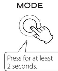
Setting mode will also end and the ordinary display will reappear if nothing is done for 10 seconds or the stop (■) button is pressed once.
