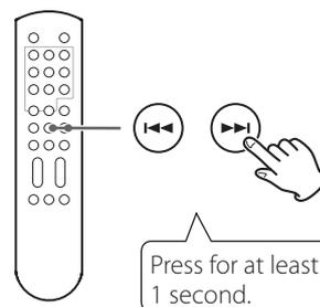
During playback, press and hold a skip (I◀◀/▶▶I) button on the main unit or the remote control until searching backward/forward starts. When you find the point where you want to listen, press the play (▶) button on the main unit or the play/pause (▶/||) button on the remote control.
