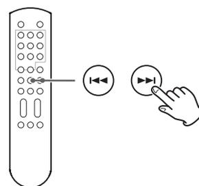
During playback, press a skip button (I◀◀/▶▶I) on the main unit or the remote control to skip to the previous or next track and start playback.
