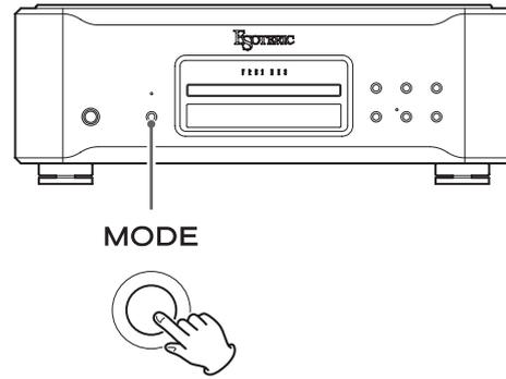
This unit can be used as a D/A converter when its input source is set to an external digital input (COAX in, OPT in or USB in).
