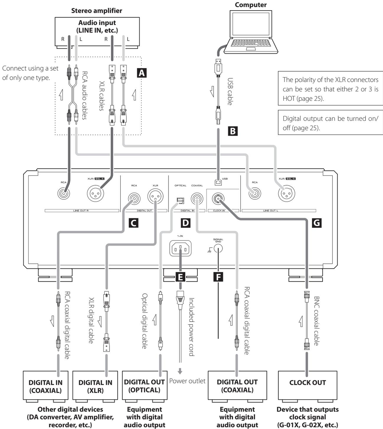
**A Analog audio output (LINE OUT) connectors**
