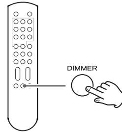
You can adjust the brightness of the main unit's display.
