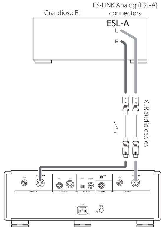
Use XLR audio cables to connect the analog audio output (XLR/ESL-A) connectors on this unit to a Grandioso F1 or other amplifier that has ES-LINK Analog (ESL-A) connectors.
