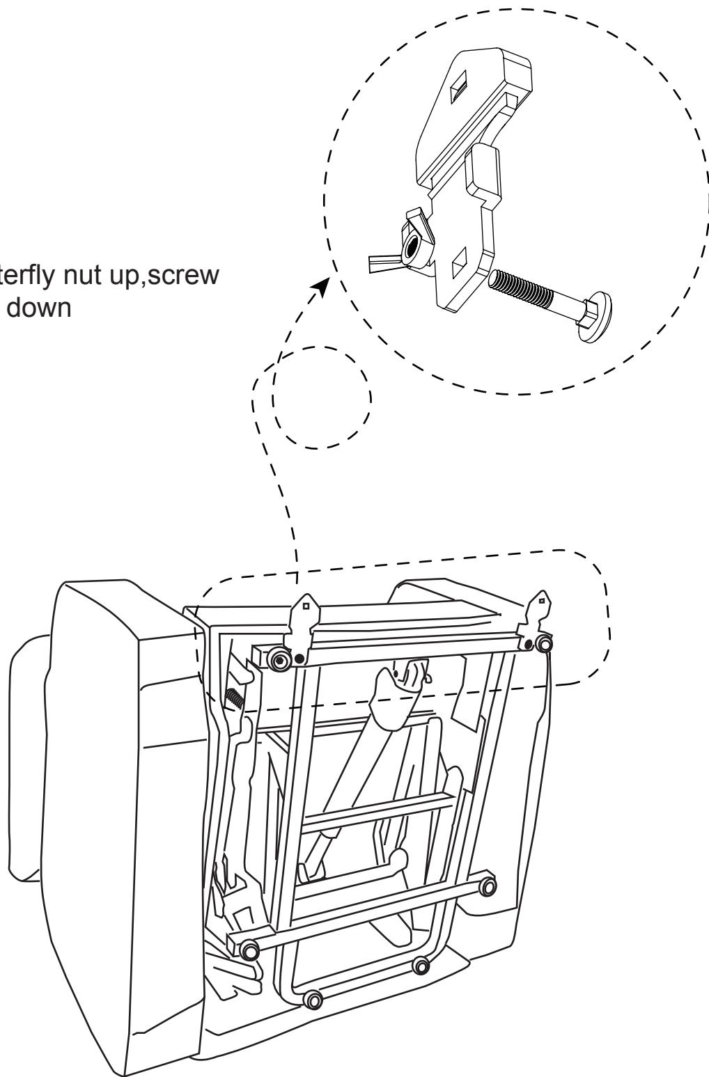
Find a small bag in the accessories box. Take out **Anti-fall Brackets\*2(E)** from the small bag. Assemble the two Anti-fall Brackets as shown on the bottom of mechanism to avoid toppling and falling.
