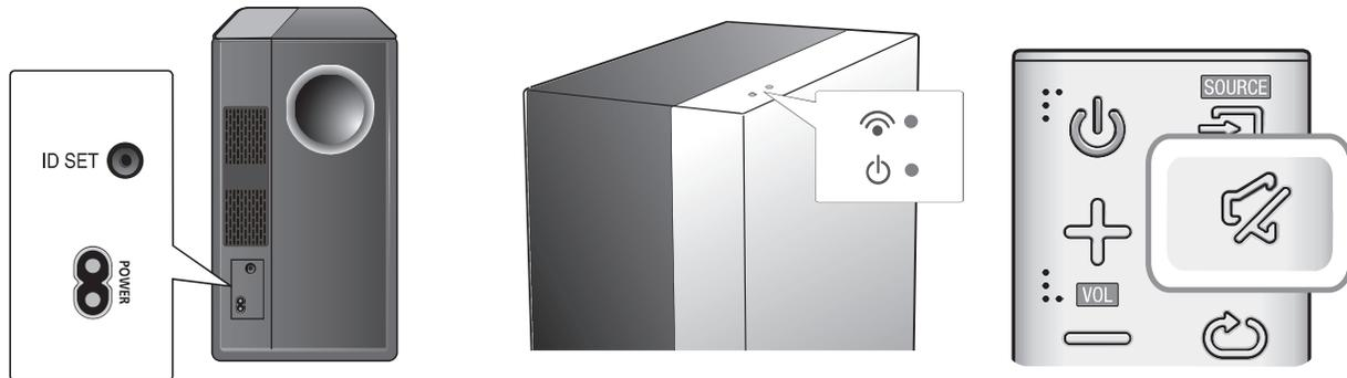
1. Plug the power cords of the main unit and subwoofer into an AC wall outlet.
