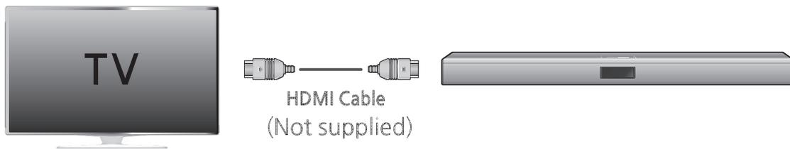
1. Connect the TV supporting ARC to the Soundbar with an HDMI cable.
