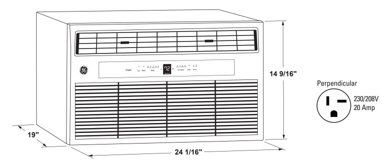
Note: When installing units in through-the-wall applications.
