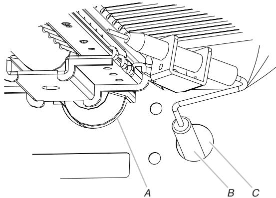
A. Broil burner orifice hole
