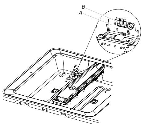
A. Oven bake burner electrode bracket
