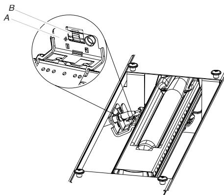
A. Oven bake burner electrode bracket
