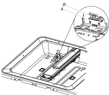
A. Oven bake burner electrode bracket
