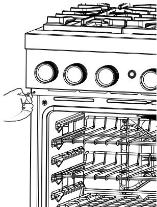
**NOTE:** Make sure to leave the door open or the control console will not rest in the side brackets properly once it is attached.
