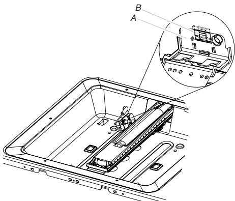
A. Oven bake burner electrode bracket
