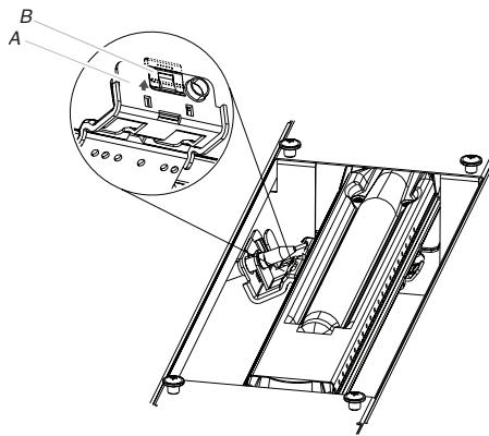
A. Oven bake burner electrode bracket
