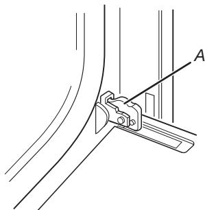
A. Oven door hinge in the locked position
