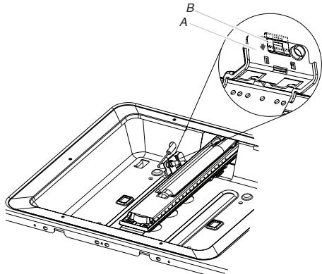
A. Oven bake burner electrode bracket
