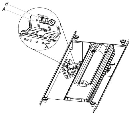
A. Oven bake burner electrode bracket
