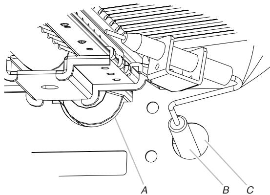
A. Broil burner orifice hole
