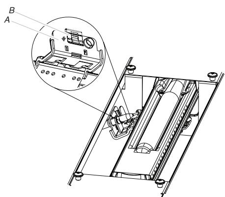
A. Oven bake burner electrode bracket
