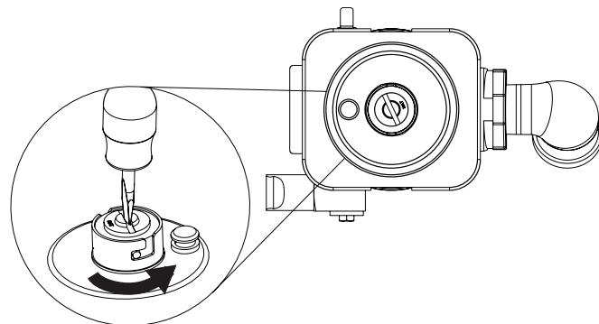
5. Turn over the gas pressure regulator cap, and reinstall on the regulator so that the hollow end faces in and the letters "NAT" are visible.
