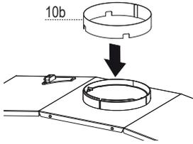
Install metal damper ring (10b) included with the Hood.
