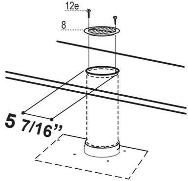
For Non-Ducted Recirculation venting route the ductwork to a location above the hood where the discharge is vented back into the room.
