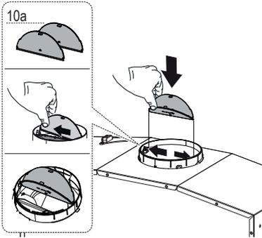
Install the damper flaps (10a) that are included with hood by snapping the tabs into place inside the top of the hood before connecting ductwork.
