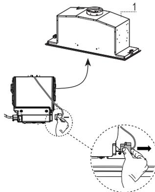
The Hood can be installed directly on the underside of the wall unit (Minimum 24" - 30" from the Cooking Surface).
