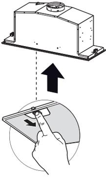
Replace the grease filters removed previously.
