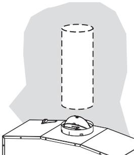
Install Roof or Wall Cap purchased separately. Connect the 6" metal ductwork to the Roof or Wall Cap and then attach ductwork. Seal with foil tape.
