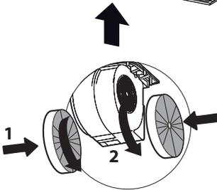
Attach each charcoal filter to the black grid on each side of the blower. Press the charcoal filter tightly to the black grid on the blower side and rotate the filter clockwise (towards the front of the insert hood) until it locks into place. Turn counterclockwise (towards the back of the insert hood) to remove.
