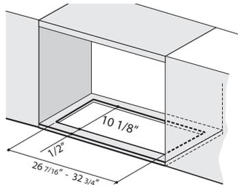
Create an opening in the bottom of the wall unit, as shown.
