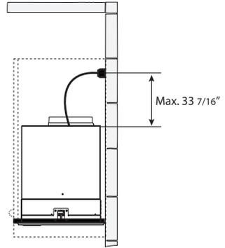
**WARNING** - "The supply cord shall be accessible for inspection after installation".
