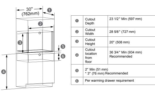
NOTE: Additional clearances between the cutouts may be required. Check to be sure the oven supports above the warming drawer location do not obstruct the required interior depth and height. See warming drawer's installation instructions for details.
