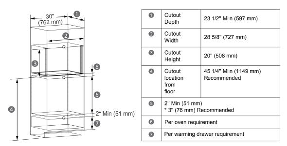
NOTE: Additional clearances between the cutouts may be required. Check to be sure the oven supports above the warming drawer location do not obstruct the required interior depth and height. See warming drawer installation instructions for details.
