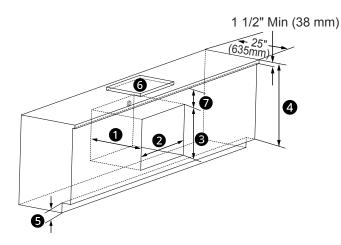
NOTE: Gas or electric cooktops may be installed over this oven. See cooktop installation instructions for the cutout size. This oven requires a separate, properly grounded 16-Amp, 120-Volt, 60Hz power supply. The cooktop requires a separate power supply. Use a 36" or wider base cabinet.
