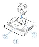
➤ After use, place the receiver into the transmitter's charging compartment ⑧ without exerting too much pressure.
