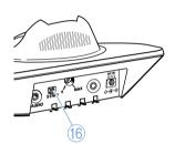
➤ Set the ST/MO switch (6) of the transmitter to MO (mono).
