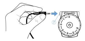
➤ Connect the 3.5 mm jack plug of the headphones to the socket ⑦ of the receiver.
