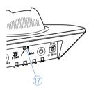
Use a screwdriver to turn the treble boost control (7) to the left or right until the sound can be heard very well.
