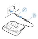
Plug the other end of the connection cable (9) into the head-phone socket on your sound source.
