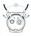
➤ Connect the fasteners of the lanyard ② to the metal ring at the rear of the receiver.
