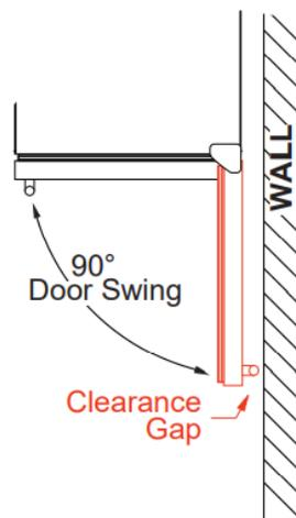
When installing with The hinge side next to a wall -Leave 1-3/4" clearance gap for cabinet handles door must be able to open a minimum of 90° .
