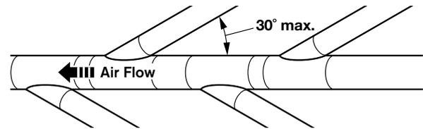
The maximum angle of each vent entering the main vent should be no more than 30°.
