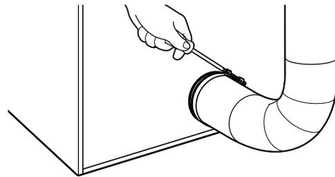
4. Make sure the vent is secured to exhaust hood with a 4" (102 mm) clamp.
