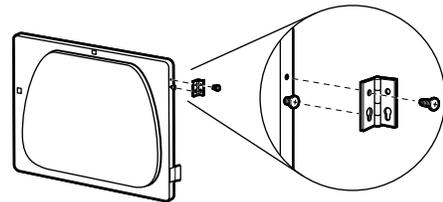
10. Remove the 4 screws that attach 2 plugs on the left side. Attach plugs to right side using the same 4 screws.
