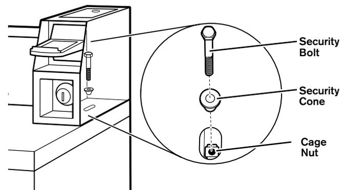
**NOTE:** Installing the security bolt provides added security, but will add to the service time when the top needs to be removed or lifted for servicing the dryer.
