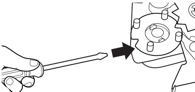
5. Place new cam (hub side down) over clock shaft. Line up flat side of shaft with flat side of cam hole. Check that drive lug is in place.
