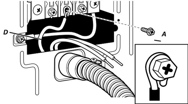
3. Connect remaining wires under outer terminal block screws (F). Squeeze hooked ends together and tighten screws. Finally, reinstall terminal block cover to dryer rear panel. Secure cover with hold-down screw. Now go to "Venting Requirements."
