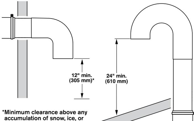
If main vent travels vertically through the roof, rather than through wall, install a 180° sweep elbow on end of vent at least 2 ft. (610 mm) above surface of roof.
