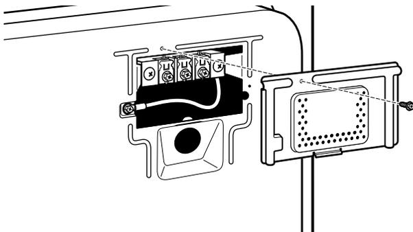
Remove hold-down screw and terminal block cover.
