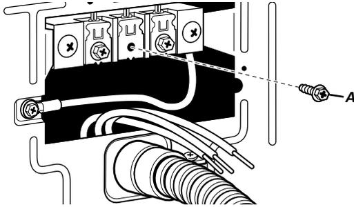
2. Place hooked end of neutral wire (white or center wire) (D) of direct wire cable under center terminal block screw (A), hook facing right. Squeeze hooked end together and tighten screw.
