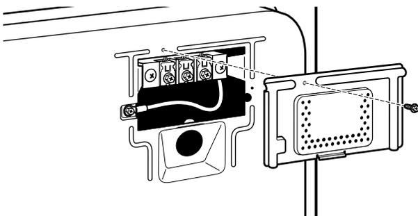
Remove hold-down screw and terminal block cover.
