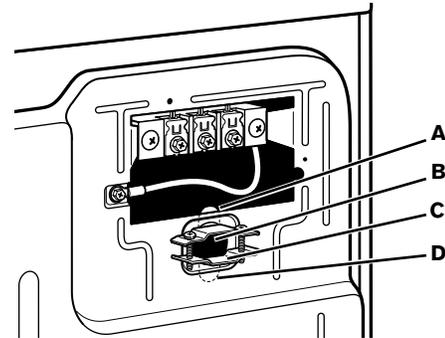
Remove the screws from a 3/4" (19 mm) UL listed strain relief (UL marking on strain relief). Put the tabs of the two clamp sections (C) into the hole below the terminal block opening (B) so that one tab is pointing up (A) and the other is pointing down (D), and hold in place. Tighten strain relief screws just enough to hold the two clamp sections (C) together.
