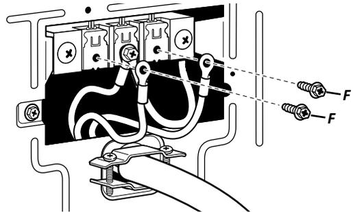
4. Connect a separate copper ground wire (G) under the green external ground conductor screw (C) to an adequate ground. Finally, reinstall terminal block to dryer rear panel. Secure cover with hold-down screw. Now go to "Venting Requirements."
