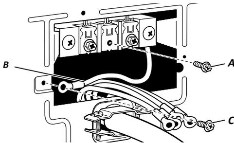
2. Connect neutral ground wire (B) and neutral wire (white or center wire) (D) of power supply cord under center terminal block screw (A). Tighten screw.
