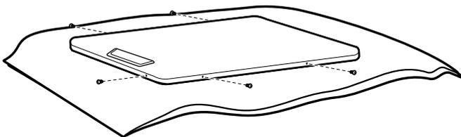
6. Holding door over towel on dryer, grasp sides of outer door and gently lift to separate it from inner door. Do not use a putty knife to pry apart. Do not pull on door seal or plastic door catch.
