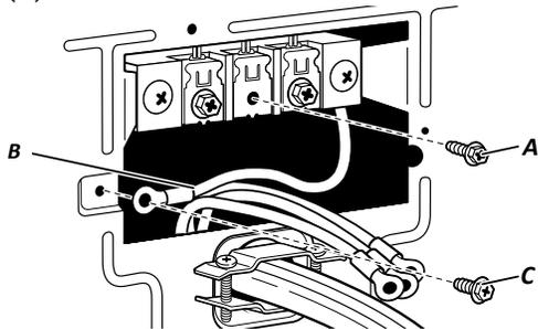
2. Connect neutral ground wire (B) and neutral wire (white or center wire) (D) of power supply cord/cable under center terminal block screw (A). Tighten screw.
