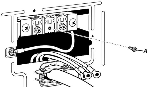
2. Connect neutral wire (white or center wire) (D) of power supply cord under center terminal block screw (A). Tighten screw.
