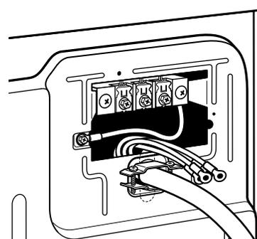
Put power supply cord through the strain relief. Be sure that the wire insulation on the power supply cord is inside the strain relief. The strain relief should have a tight fit with the dryer cabinet and be in a horizontal position. Do not further tighten strain relief screws at this point.
