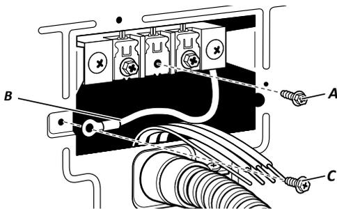
2. Connect neutral ground wire (B) and place hooked end (hook facing right) of neutral wire (white or center wire) (D) of direct wire cable under center terminal block screw (A). Squeeze hooked ends together and tighten screw.
