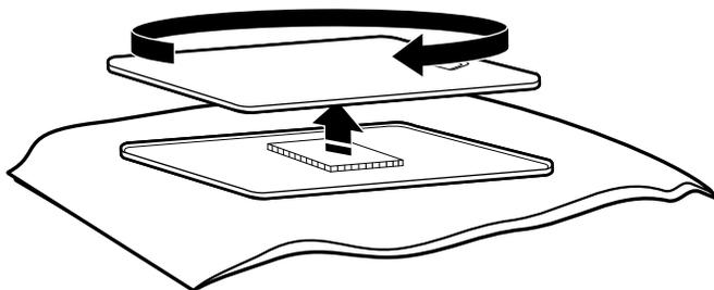
7. Be certain to keep cardboard spacer centered between doors. Reattach outer door panel to inner door panel so handle is on the side where hinges were just removed.
