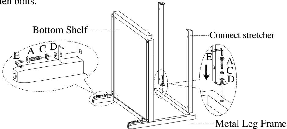
**STEP 3:** Attach another metal leg frame to connect stretchers and bottom shelf by using 4 bolts(A), lock washers(C) and flat washers(D). Do not completely tighten bolts.
