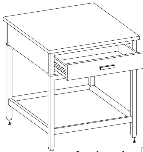
Leveler on legs Adjust the leveler when necessary
