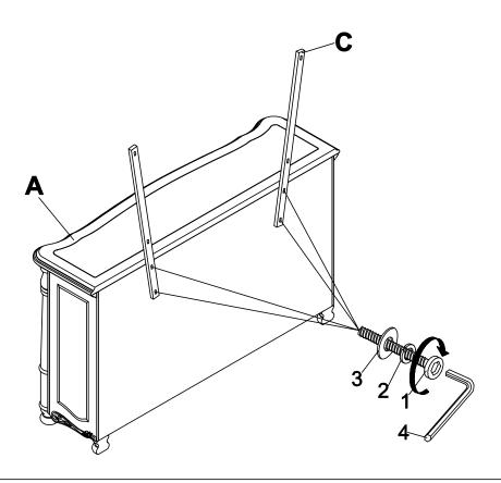
STEP 2 Assemble support (C) with mirror (B) using Allen Key (4) with hardware1,2, and 3.
