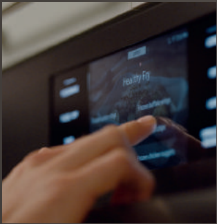
7" LCD Touch Control Panel with Guided Cooking
