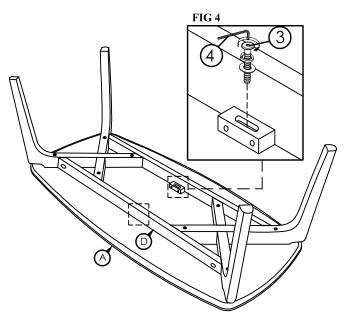
Step 4 Tighten both Leg Support (D) to Table Top (A) by using JCBC Bolt with washer (3) and Allen Key (4) into the wooden block of Leg Support (D) as shown on FIG 4.
