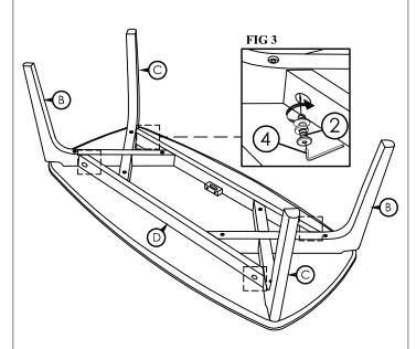
Step 3 Align both Leg Support (D) into the designated hole at both of the Table Leg Left & Right (B & C) by using JCBC Bolt with washer (2) and Allen Key (4) as shown on FIG 3.
