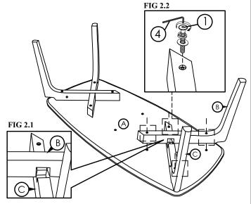
Step 2.1 Repeat Step 1.1 for the next Table Leg Left (B) & Table Leg Right (C) as shown on FIG 2.1.
