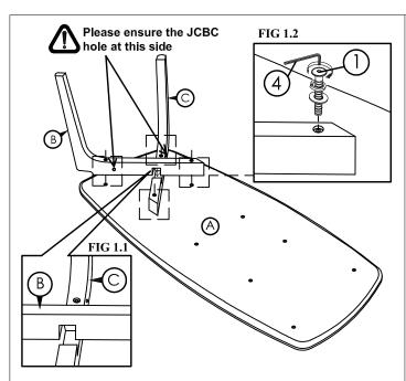
Step 1.1 Cross over Table Leg Left (B) to Table Leg Right (C) as shown on FIG 1.1.
