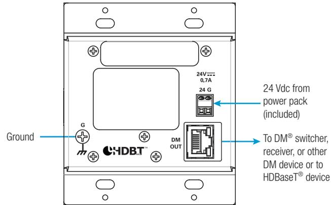
**NOTE:** The DM OUT port is a Power over DM (PoDM) and HDBaseT® PoE (Power over Ethernet) powered device (PD) port. To receive PoDM or HDBaseT PoE, the DM-TX-200-C-2G requires a connection to a DigitalMedia™ switcher or other equipment that has a PoDM or HDBaseT PoE power sourcing equipment (PSE) port. Any wiring that is connected to a PoDM or HDBaseT PoE PSE port is for intrabuilding use only and should not be connected to a line that runs outside of the building in which the PSE is located.
