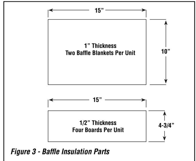
**Figure 3 - Baffle Insulation Parts**
