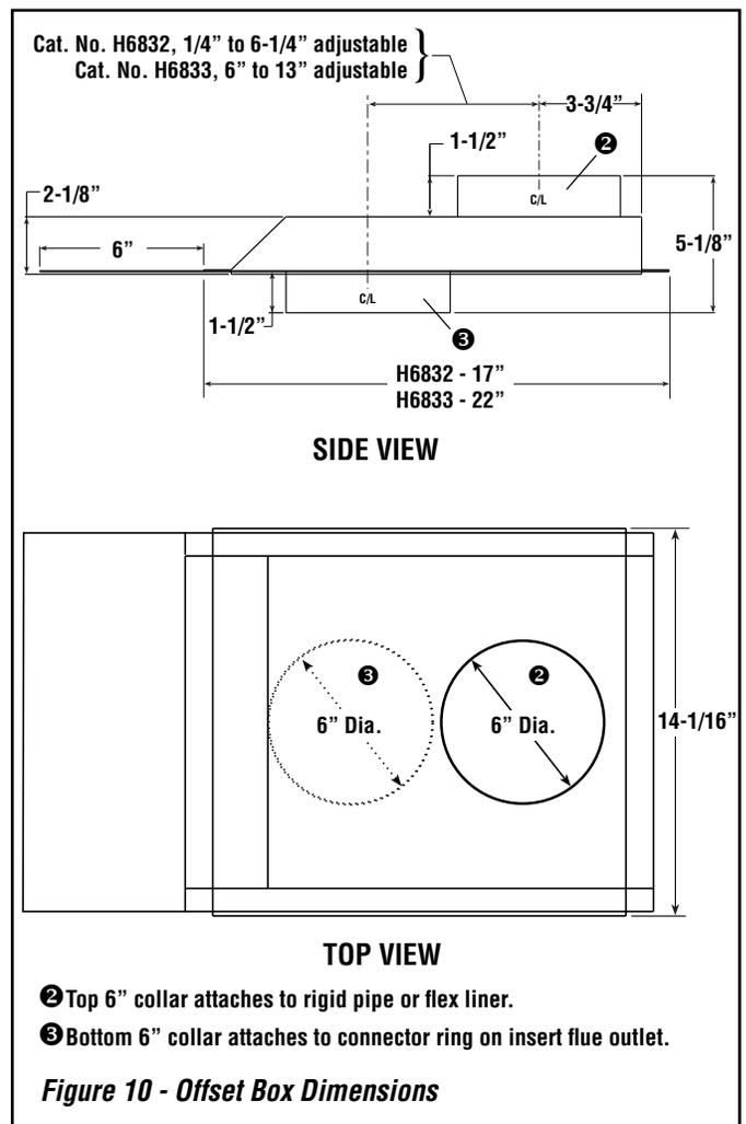
Figure 10 - Offset Box Dimensions
