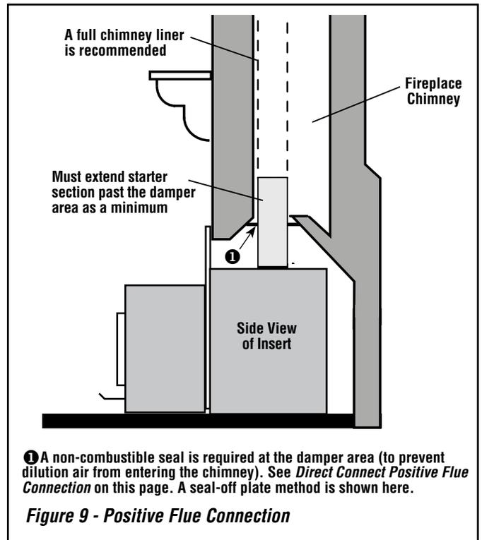
Figure 9 - Positive Flue Connection
