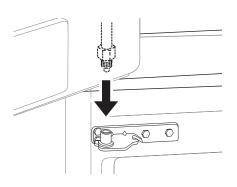
2 Fit the hinge ① over the hinge lever latch ② and slot it into place. Rotate the lever ③ clockwise and fasten the hinge.
