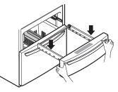
**2** Pull the drawer open to full extension. Lower the basket onto the rails.
