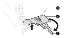
**3** Lift the door from the middle hinge pin and remove the door.
