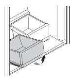
**3** To reassemble, slightly tilt up the front, insert the crisper into the frame and push it back into place.
