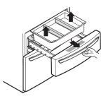
**2** Hold both sides of the door and remove it from the rails.
