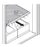
**2** Pull out the crisper to full extension, lift the front up, and pull straight out.
