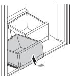
**4** Insert the cover into the refrigerator with both hands and lower it onto the guides.
