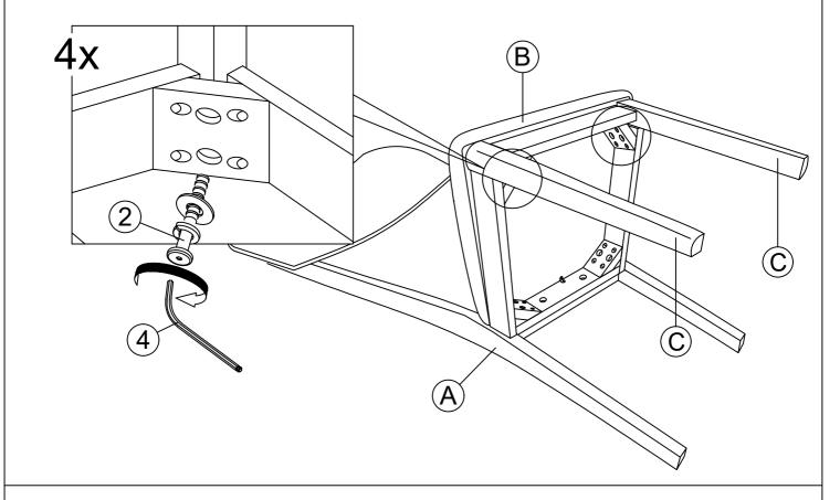
STEP 4: To level the chair, stand the chair up on a flat surface and tighten all the bolts by using Allen Key (4).
