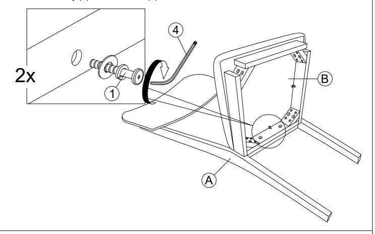
STEP 2 :Attach the seat frame with cushion (B) with the back legs of the chair back (A) by using the Allen Key (4) with hardware (3).
