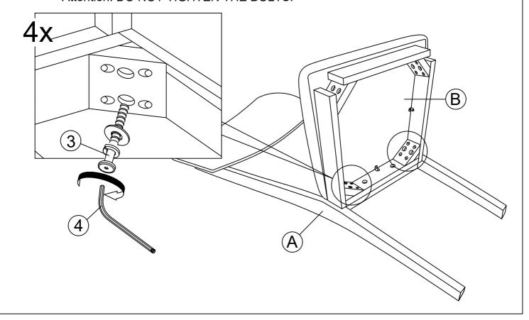
STEP 3 : Assemble the legs (C) with the seat frame with cushion (B) by using Allen key (4) with hardware (2).
