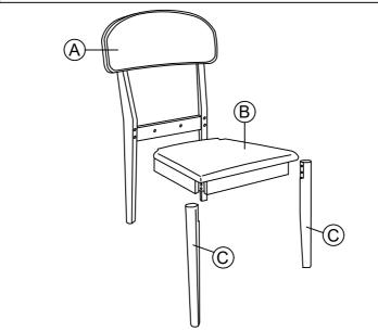
STEP 1 : Assemble the seat frame with cushion (B) with the chair back (A) using the Allen Key (4) with hardware (1).
