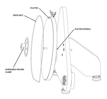
After placing the record on the platter, it is necessary to tighten the screw-able record clamp (6) onto the platter spindle.
