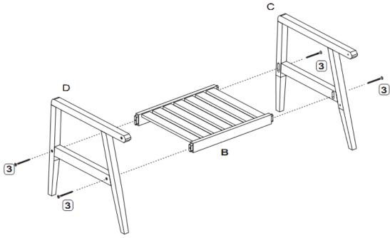
STEP 2: Installation top frame by screws. Using the Allen key to tighten all bolts.
