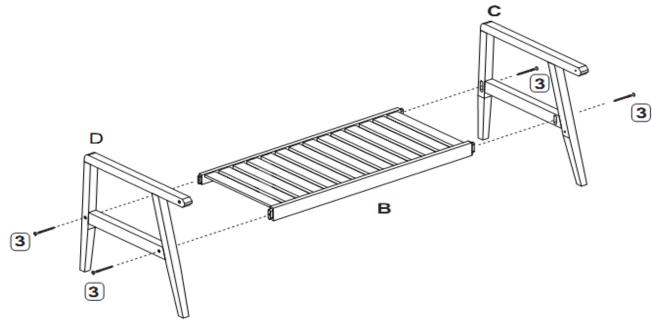
STEP 2: Installation top frame by screws. Using the Allen key to tighten all bolts.
