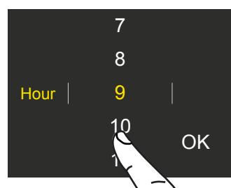
**D)** Scroll up / down to set the hour and then press ok.
