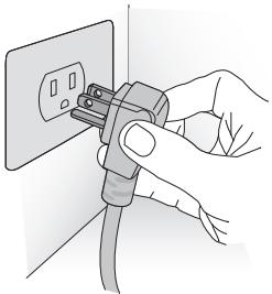
The appliance operates at 115 V AC, 60 Hz and is equipped with a power supply cord with a 3-prong grounded plug, which must be connected to a corresponding 3-prong (15 Amp) grounding-type wall receptacle.
