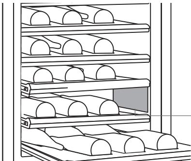
Position of the serial number inside the compartment.
