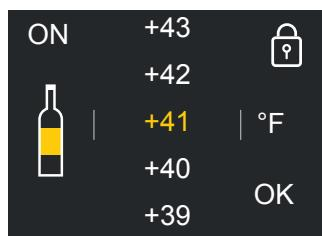
If the icon function is touched and a specific function is set, the yellow padlock will be seen closed and it won't be possible to change the temperature of the compartments as long as the function won't be completed or if it is manually deactivated as long as the function is active.
