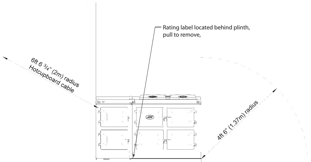
The mains supply connect point must be within the zones shown
