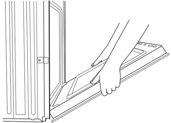
5. Using two hands, grasp the edges of the oven door. Lift and pull the oven door toward you to remove. You may need to gently shift door from side to side as you pull.
