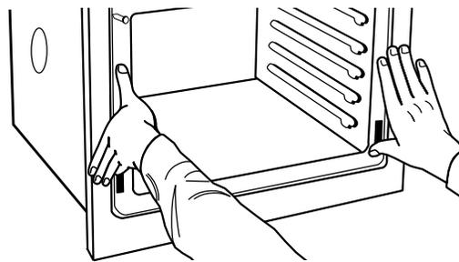
3. Push oven completely into the cabinet and center the oven into the cabinet cutout.
