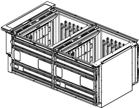
2. Install a foot on the left rear spacer using a #8-18 x ¾" screw.
