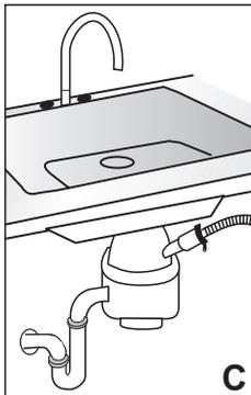
Every disposal has a hook up for a dishwasher; consult your disposer manual for correct connection. (Figure **C**)
