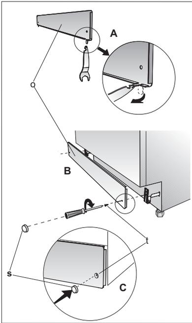
Lock the toe kick brackets as shown with the plastic tab in the figure C by pushing the plastic tab on the dishwasher into the teeth of the bracket (C).
