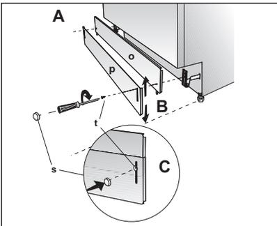
If the enclosure height is above  $33 1/16"$  (840mm) use "o" and "p" labelled toe kicks together. Make sure the slotted toe kick "p" is on the outside so you can adjust height of the toe kick. Installation should be done following the steps illustrated in the figures A, B and C respectively.
