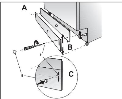
If the enclosure height is above  $34 1/4"$  (870mm) use "o" and "r" labelled toe kicks together. Make sure the slotted toe kick "r" is on the outside so you can adjust height of the toe kick. Installation should be done following the steps illustrated in the figures A, B and C respectively.
