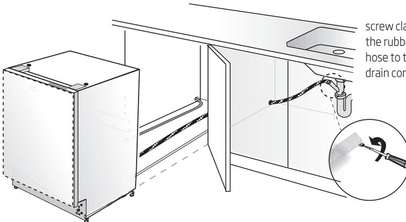
screw clamp to secure the rubber connection hose to the plumbing drain connection.
