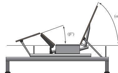
normal operating use. Normal operating use is defined as the following: Adjustable foundation is to be operated with a mattress and load. Testing procedures require lifetime cycle tests with up to 120 kg distributed load. The angle (designated "a" in figure 1) between the back section and the flat section for various configurations of the mattress support platform shall be  $\pm 3^\circ$ , which translates to a tolerance of up to  $1\frac{1}{2}''$ .
