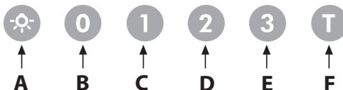
• The appliance has the **INTENSIVE** speed function, press key **E** for two seconds and it will be activated for 10 minutes after which it will return to the previously set speed. When the function is active the LED flashes. To interrupt it before the 10 minutes have expired press key **E** again.
