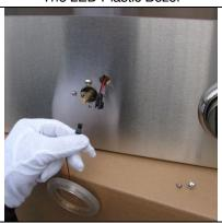
Disconnect the Wire and Change New LEDs
