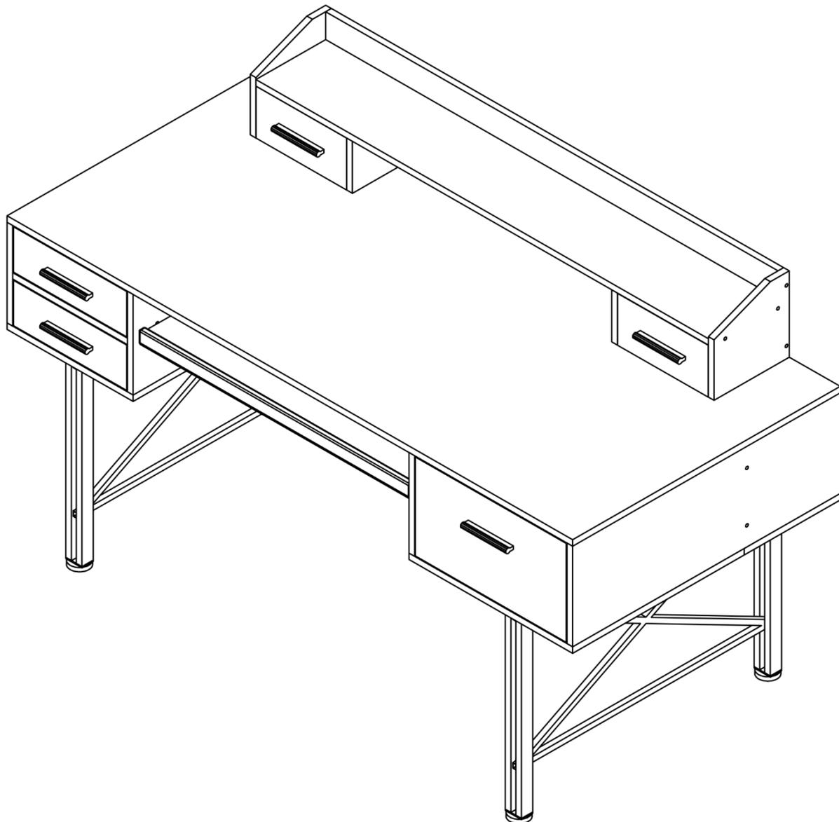
\*\* Do not fully tighten screws until fully assembled \*\*\*
