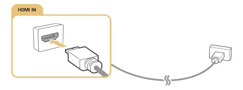
Set Edit Device Type to DVI PC for a computer connected with a HDMI-to-DVI cable, and PC for a computer connected with HDMI cable. Also, set Edit Device Type to DVI Devices for an A/V device with a HDMI-to-DVI cable.
