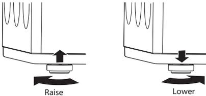
2. Adjust the leveling feet. Turn clockwise to raise the washer or counterclockwise to lower it.
