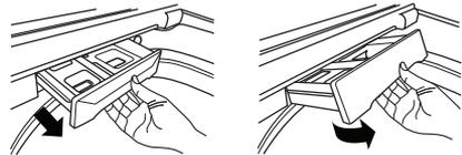
1. Remove the drawer by pulling it straight out until it stops. Lift up on the front of the drawer and pull it completely out.
