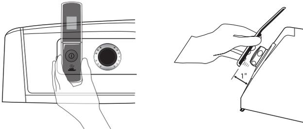
**HOLD** the mouthpiece of your phone over the power button, when instructed to do so by the call center, no more than one inch from (but not touching) the machine.
