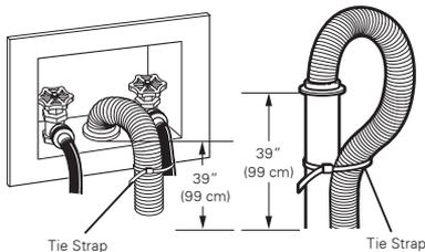
fasten the drain hose to one of the water hoses with the tie strap (ribbed side on inside).
