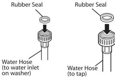
1. Inspect the threaded fitting on each hose and make sure there is a rubber seal in place in both ends.
