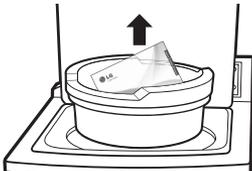
3. Carefully remove the two foam pads which cover the top sides of the tub guide, making sure not to leave behind any pieces of the foam.
