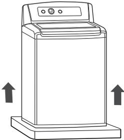
If you must lay the washer down to remove the base packaging materials, always protect the side of the washer and lay it carefully on its side. DO NOT lay the washer on its front or back.
