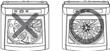
3. To make sure that the washer is properly level, open the lid and look from above to see if the tub is centered. If the tub is NOT centered (as shown in the drawing with the X through it), readjust the front feet. If you have a level, check your washer with the level.
