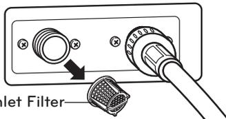
1. Turn OFF both water faucets completely. Unscrew the hot and cold water lines from the back of the washer.
