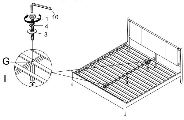
STEP 6 Assemble Slats (G) to the side rails (C) by using a screw drive with hardware 9.
