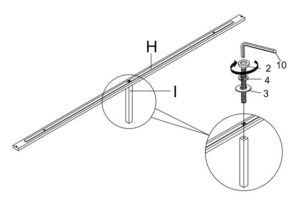
STEP 4 Assemble Slats support cross bar (H) to Headboard(A) and Footboard (B) by using a screw drive with hardware 9
