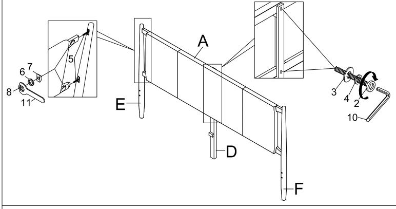
STEP 2 Assemble side rails (C) to HB legs (E & F) and Footboard (B) by using open wrench (11) with hardware 5, 6, 7, and 8.
