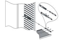
To remove the shelves out of the rail pull each shelf approximately 100% out. Use a long flat screwdriver to press down the right plastic notch as shown in Figure A and at the same time lift the left plastic notch as shown in Figure B. Then proceed to pull out the shelf slowly. Contact our service department if assistance is needed.
