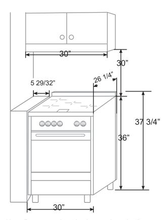
Note: Range can be raised approximately 1" (2.5 cm) by adjusting the leveling legs. The front of door and drawer may extend farther forward depending on styling.
