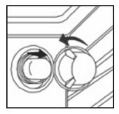
3. Remove the burned-out bulb from the socket.
