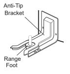
Making sure the anti-tip bracket is installed:
