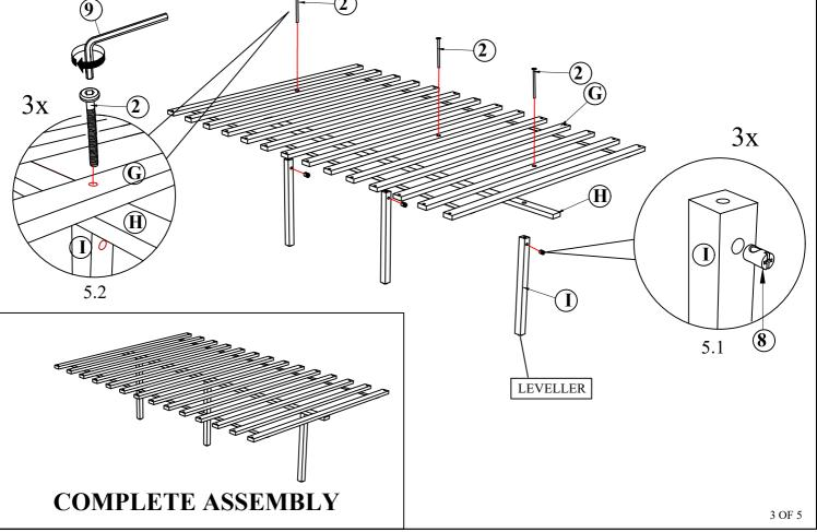
**STEP 6**: Attach and align Assembly slat (G) on into a bed frame as shown.
