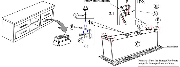
**STEP 3.1**: Pull the drawer and take out the Leg (K), (L)&(M). Attach the Chrome metal leg (K) at the bottom Storage side rails ( J ). Used Pan head chipboard screw( 6 ) and Tighten as shown.
