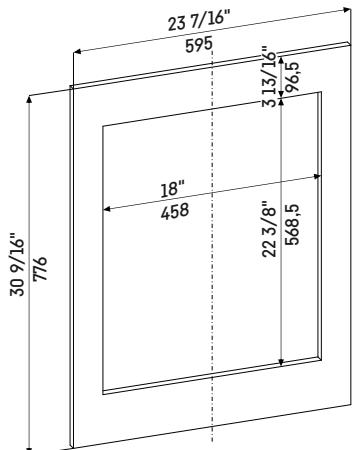
The door should be at least 5/8 in. (16 mm) thick to allow the connecting rails to be fastened to it. The maximum thickness of the door panel can be 3/4 in. (19mm).
