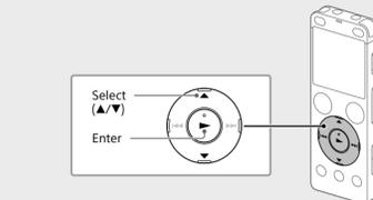
When you turn on your IC recorder for the first time, the "Configure Initial Settings" screen appears on the display window. You can then select the display language, set the clock, and turn on/off the beep sound.
