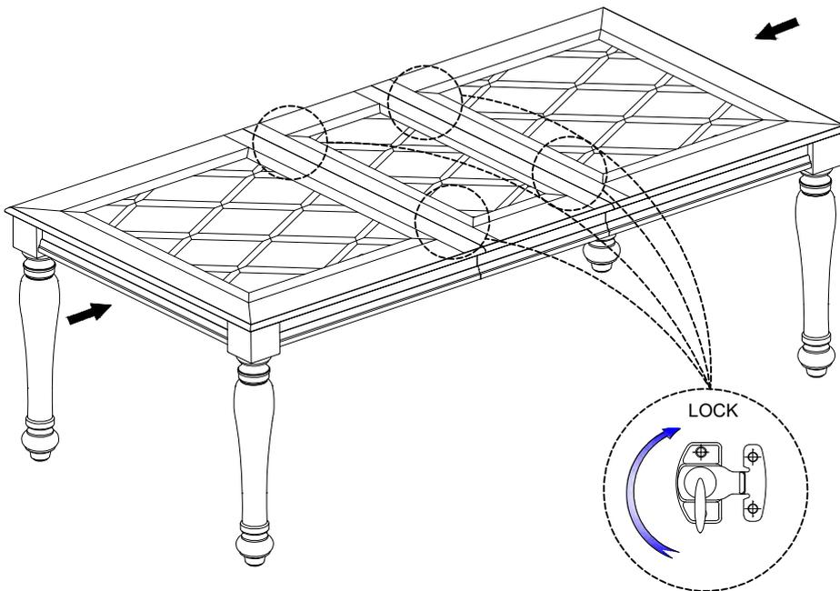
Lock the locking mechanism from underneath the table top.
