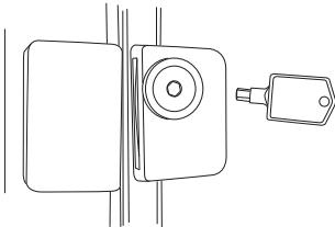
The key for the spring-loaded lock is automatically ejected—key will not remain in lock in either the open or closed position.
