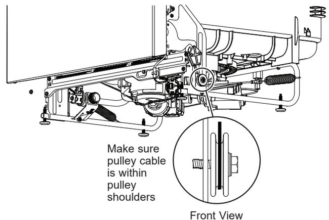
Make sure pulley cable is within pulley shoulders
