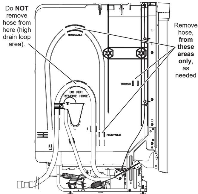
The molded end of the drain hose will fit 5/8" through 1" diameter inlet ports on the air gap, waste tee or disposer.
