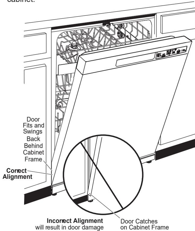
**Tip: Prevent unnecessary service charges for panel damage or wash performance.**
