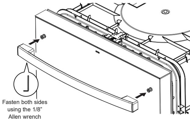
Fasten both sides using the 1/8" Allen wrench
