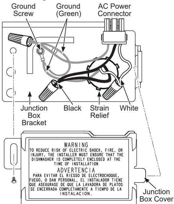
**NOTE:** All ground screws, brackets and wires must remain intact.
