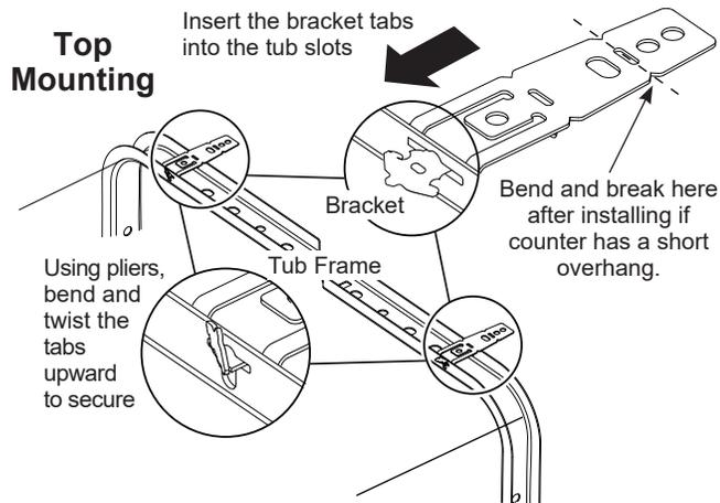
Using pliers, bend and twist the tabs upward to secure as shown.
