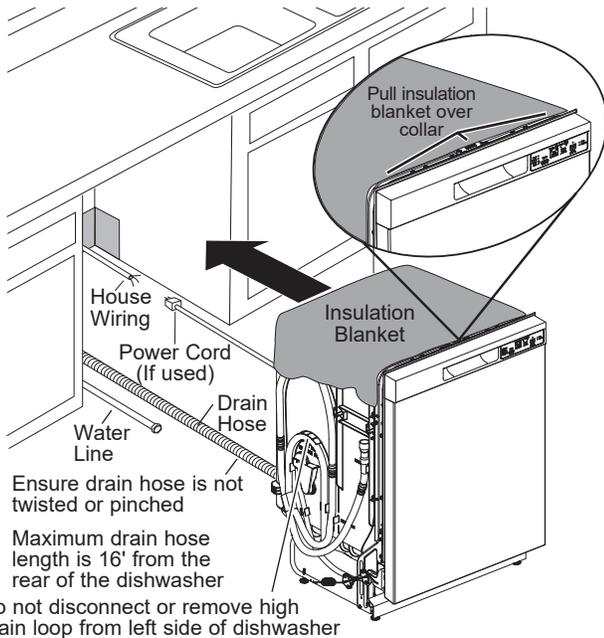
**Tip: Prevent unnecessary service call charges for fill, drain or noise concerns.**
