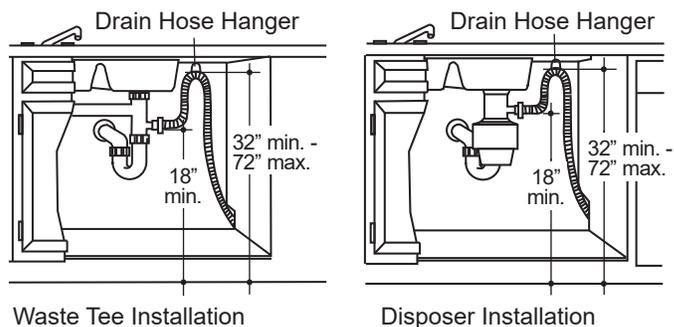
**IMPORTANT** – When connecting drain line to disposer, check to be sure that drain plug has been removed. **DISHWASHER WILL NOT DRAIN IF PLUG IS LEFT IN PLACE.**
